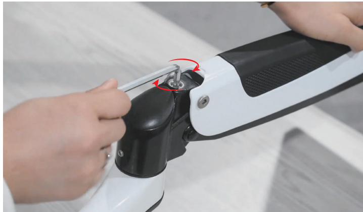
The wrench adjusts the inner damping screw to raise and lower the arm
